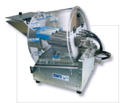
The MAFU Drum is a disentangling unit that allows the gentle and efficient disentangling and separation of small parts, for example, springs, pins, bent-wire parts, and similar, from goods delivered in bulk.
