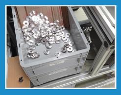
Automating the process of feeding blank parts into the Affolter machine would optimise the productivity and efficiency of the cell.
