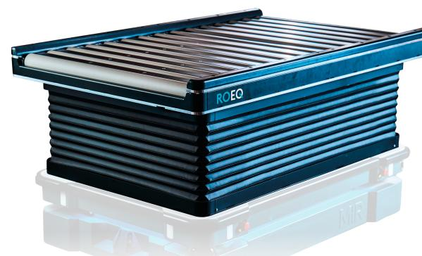
The ROEQ TR500 Auto allows you to use your MiR500, MiR600, MiR1000 and MiR1350 robots to transfer heavy goods between conveyor stations at different heights. It has a built-in scissor mechanism for automatic height adjustments. Using the ROEQ Assist software tool for set up, you can easily program the pick-up and delivery points in the MiR GUI. With a large stroke – 240mm/9.4" – it gives you the flexibility to adjust to your existing setup.
